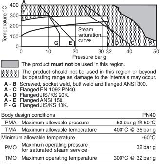
0°C Minimum operating temperature Note: For lower operating temperatures consult Spirax Sarco Designed for a maximum cold hydraulic test pressure of 75 bar g
