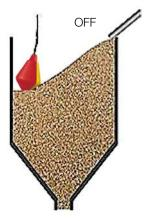
When the high level is reached, the level sensor tilts and stops filling the silo.
