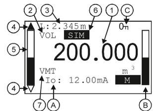
Measurement displaying with the NRM-300P display unit
