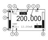
Measurement displaying with the NRM-300P display unit
