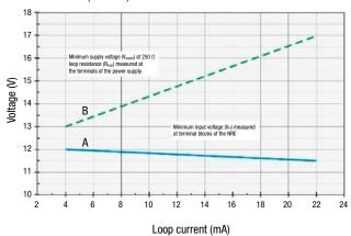
Line "A": minimum voltage at the input terminals of the device
